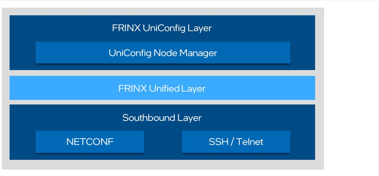
**Figure 1.** UniConfig's three layers
