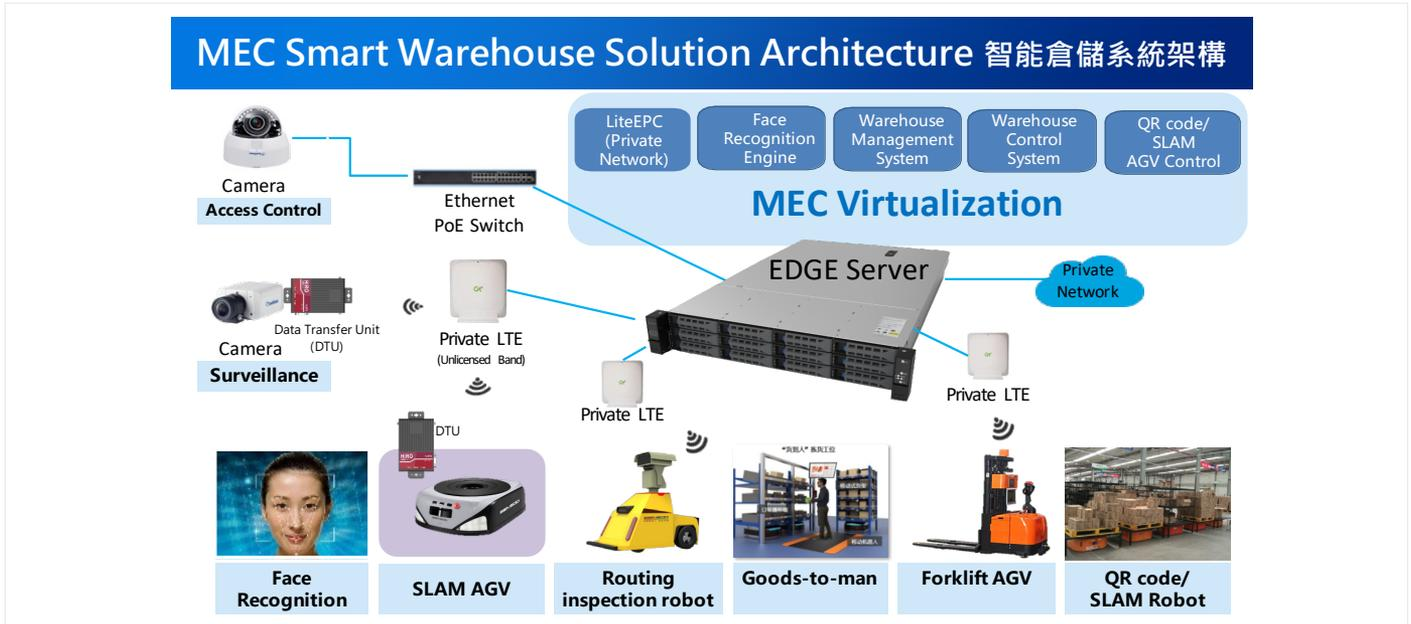
Figure 2. MEC-based smart warehouse solution architecture.<sup>1</sup>
