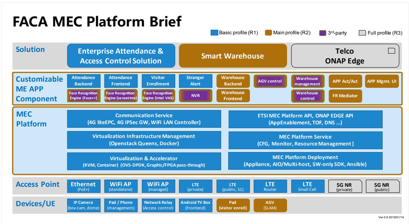
Figure 1. Block diagram of MEC solution developed by the Foxconn Advanced Communication Academy (FACA).<sup>1</sup>
