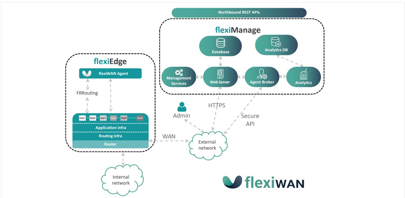
Figure 2. flexiWAN SD-WAN architecture including the flexiEdge and flexiManage software.<sup>2</sup>
