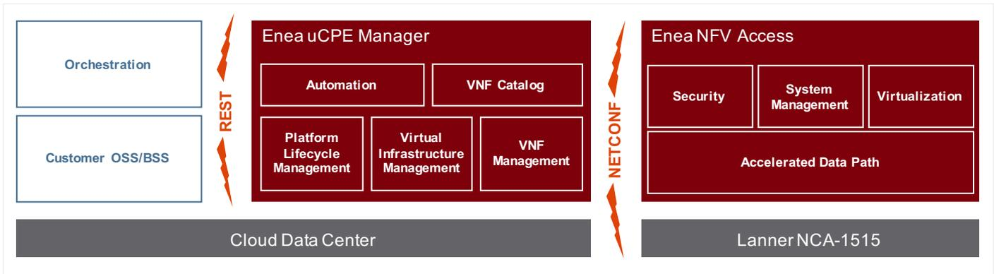
Figure 1. Enea NFV Access block diagram.<sup>1</sup>
