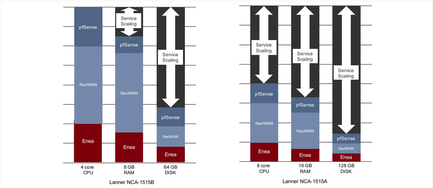
**Figure 4.** Comparison of resources available on two Lanner uCPE platforms for scaling the open-source, firewall-protected SD-WAN application.
