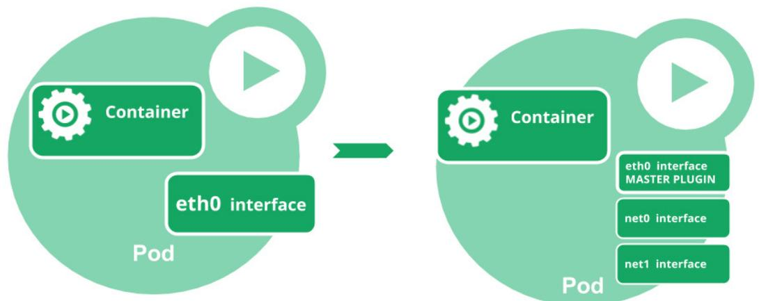
Figure 3. Before and after adding a Multus Plugin to the CNI (Image Source [here](#))
