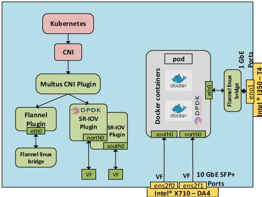
Figure 4. Mutus plugin allowing for 2 types of plugins per pod: Flannel and SR-IOV plugins
