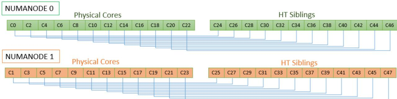
**Figure 5.** CPU Configuration of the Kubernetes Host Machines used in the solution
