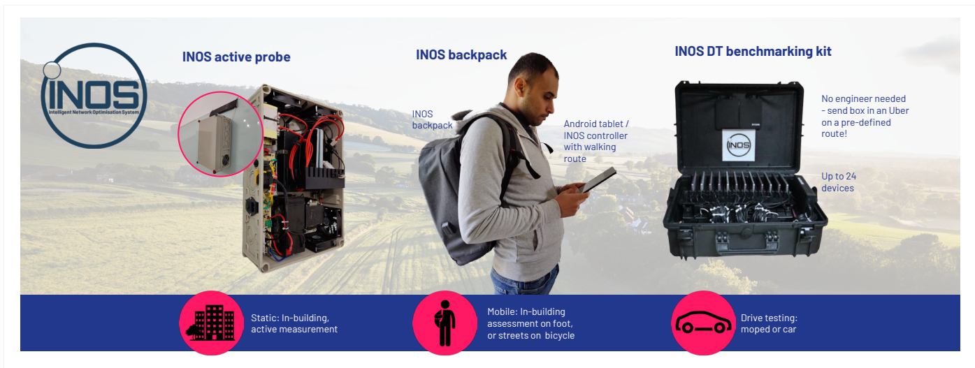
Figure 2. Three form factors of the INOS radio testing system. Photo by Digis Squared
