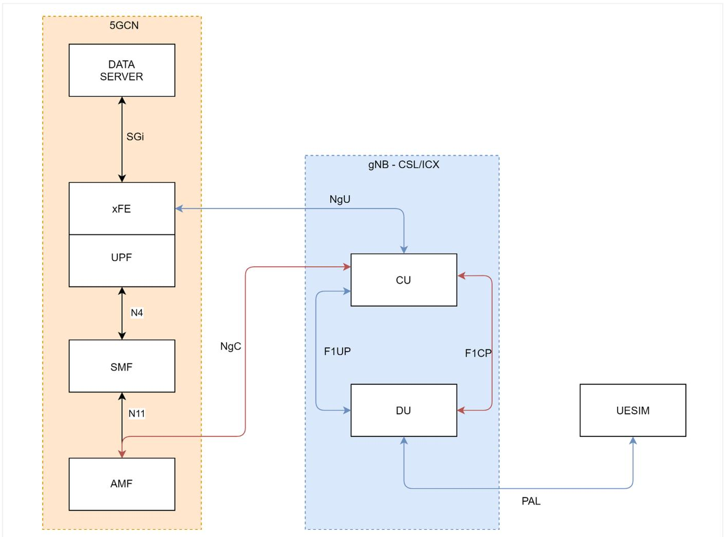
Figure 1. End-to-end 5G SA PAL network architecture.
