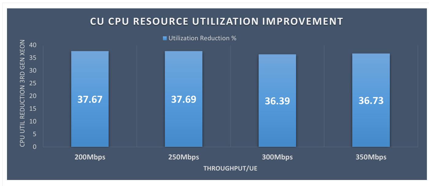
Figure 5. Average CU CPU utilization reduction in DUT1 vs. baseline for a six-cell configuration with 23 UEs (higher is better).
