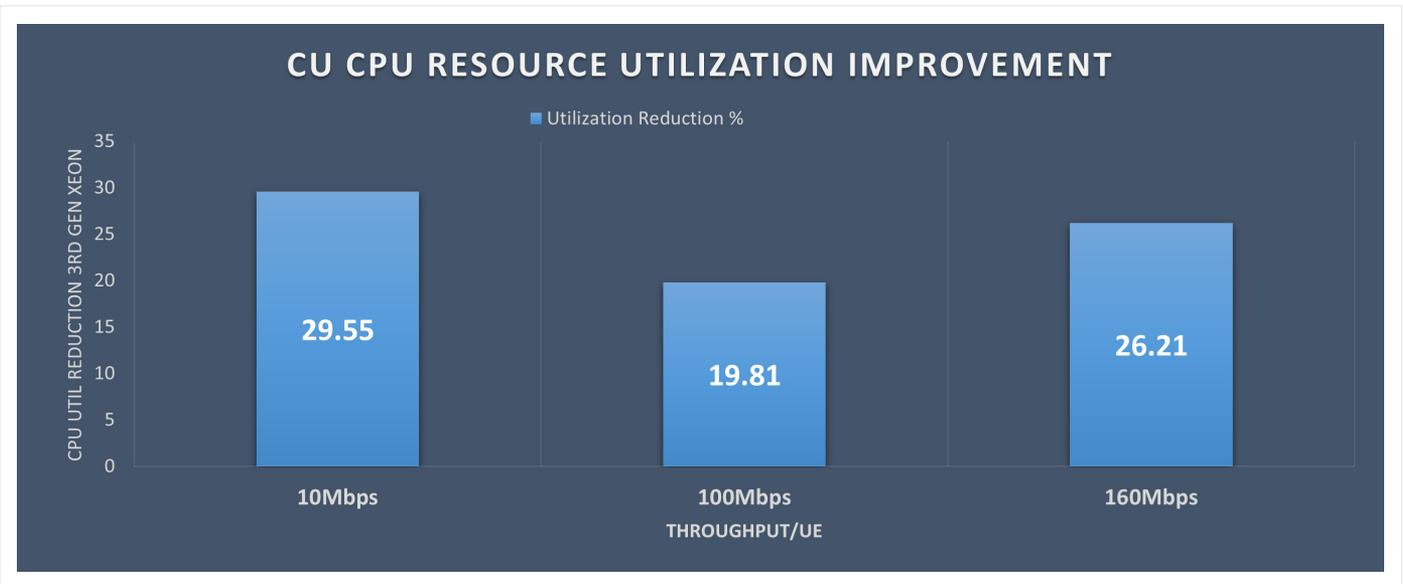
Figure 9. Average CU CPU utilization reduction in DUT1 vs. baseline in a six-cell configuration with 60 UEs (higher is better).
