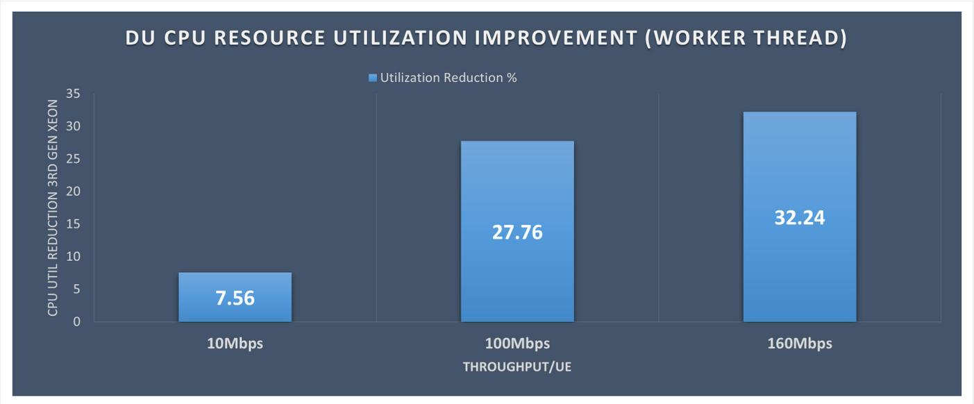
Figure 8. DU Worker Thread CPU Utilization reduction in DUT1 vs. baseline in a six-cell configuration with 60 UEs (higher is better).
