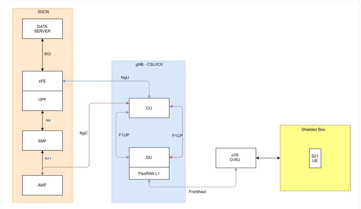
**Figure 2.** End-to-end 5G SA OTA network architecture.
