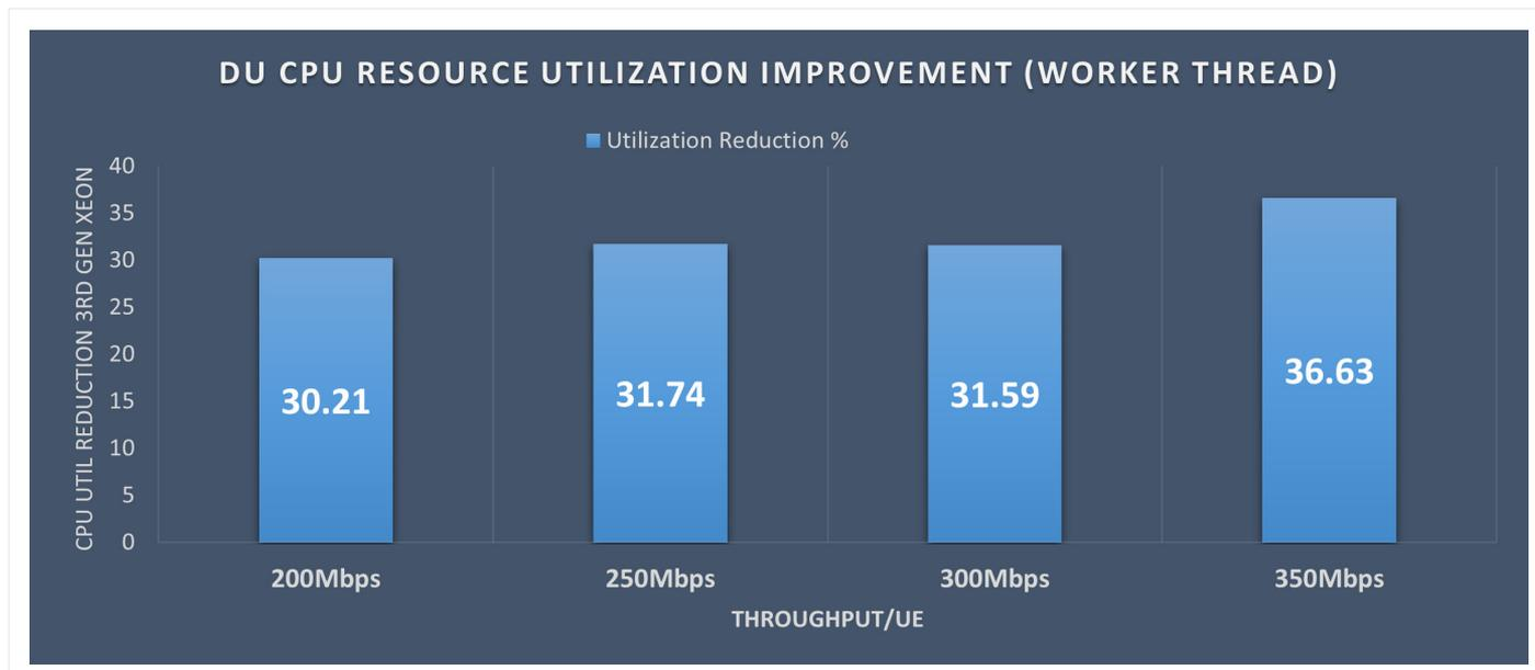
Figure 4. DU worker thread CPU utilization reduction in DUT1 vs. baseline for a six-cell configuration with 23 UEs (higher is better).
