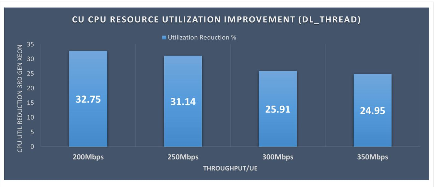
**Figure 6.** CU downlink thread CPU utilization reduction in DUT1 vs. baseline for a six-cell configuration with 23 UEs (higher is better).
