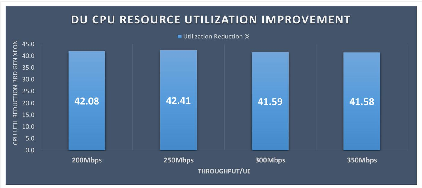
Figure 3. Average DU CPU utilization reduction in DUT1 vs. baseline for a six-cell configuration with 23 UEs (higher is better).
