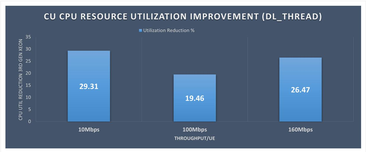
**Figure 10.** CU downlink thread CPU utilization reduction in DUT1 vs. baseline in a six-cell configuration with 60 UEs (higher is better).
