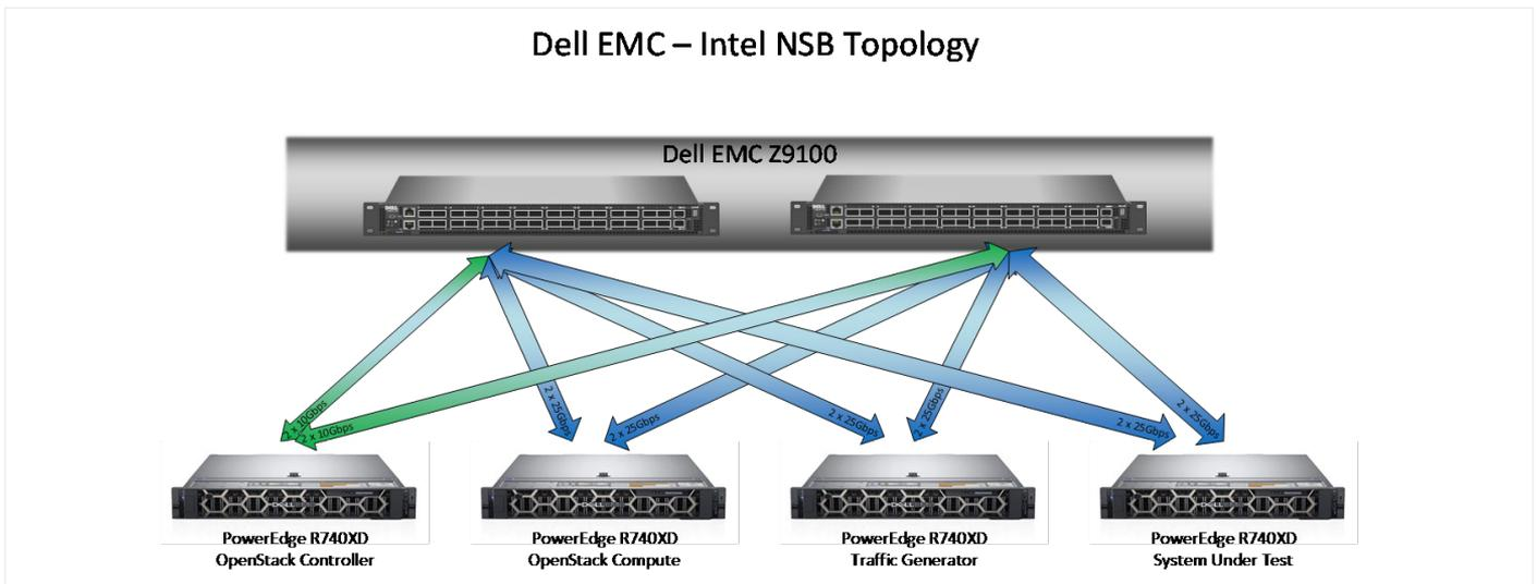
Figure 1. Dell EMC and Intel NSB Topology<sup>1</sup>
