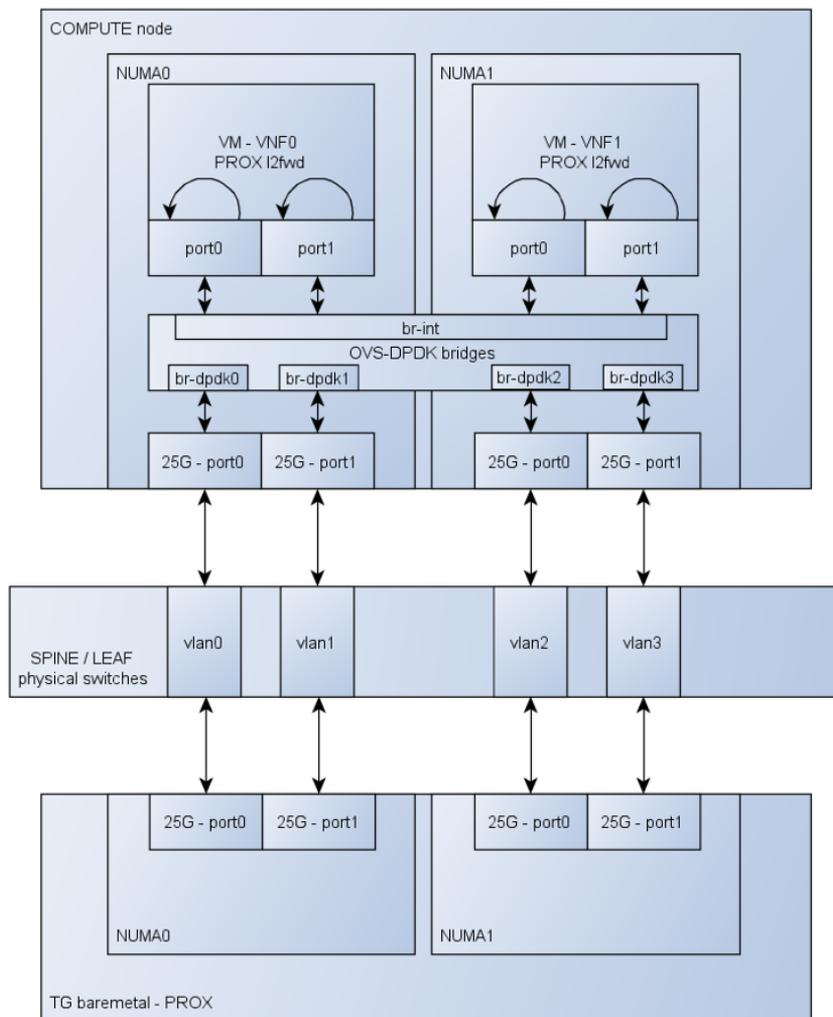
Figure 2. Logical connections between traffic generator and the OpenStack compute node.<sup>1</sup>
