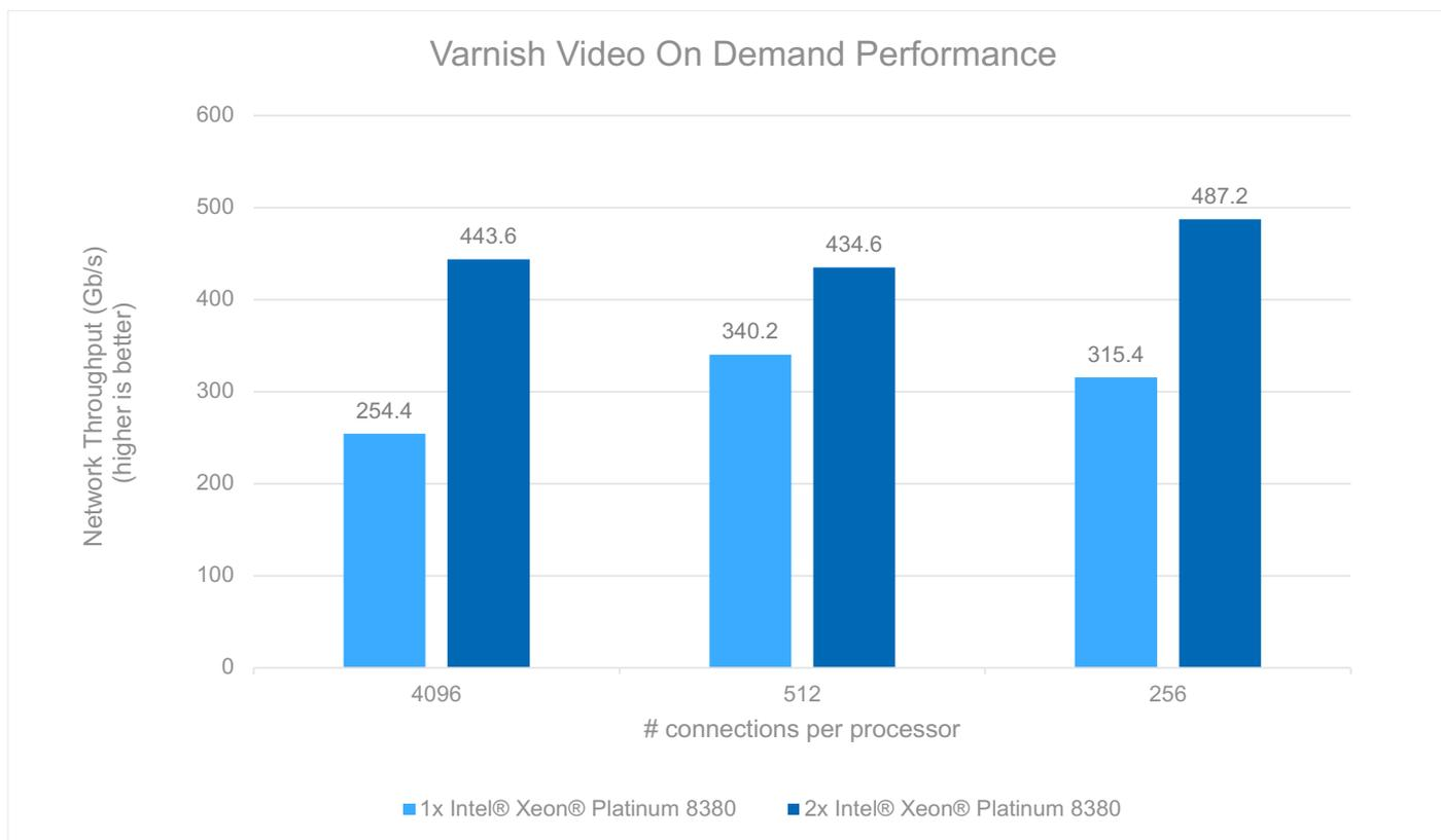
**Figure 5.** VoD performance for Varnish CDN software running on single and dual socket servers. The highest performance came with 256 connections.
