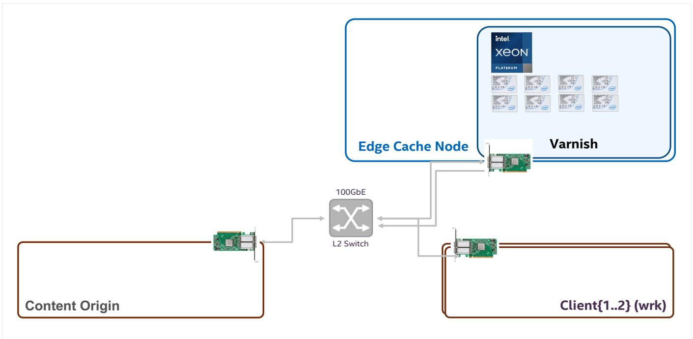
Figure 2. Single processor CDN test configuration.
