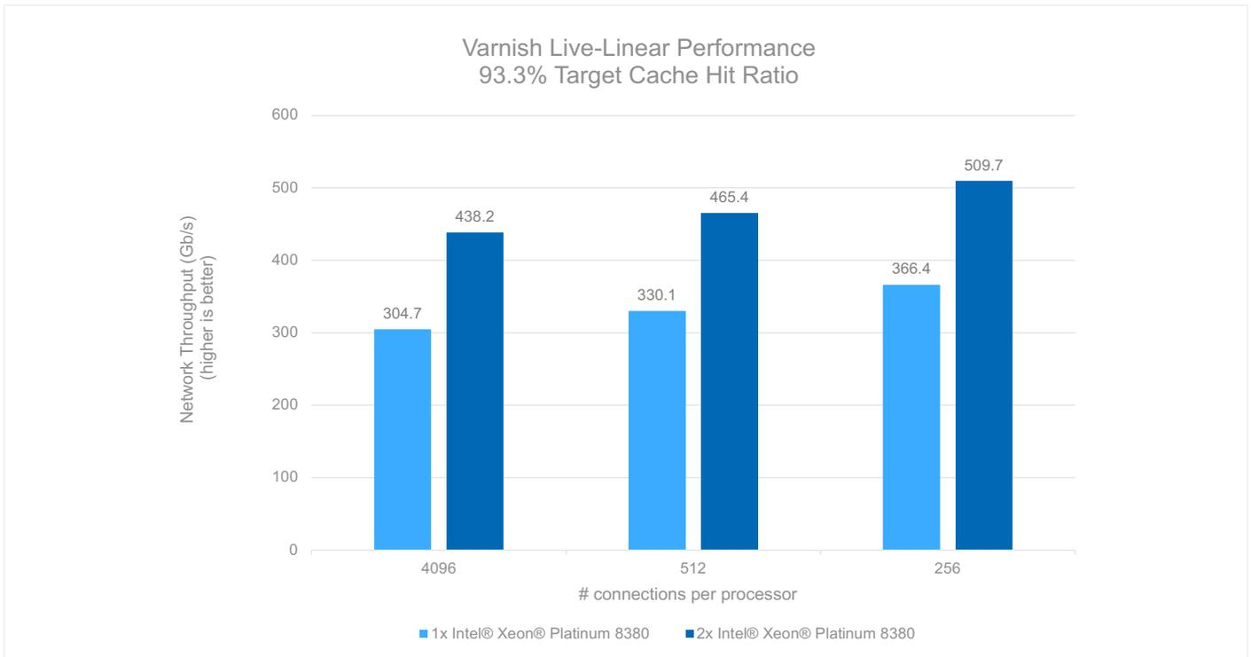
Figure 4. Live-linear video performance for Varnish CDN software running on single and dual socket servers. The highest network throughput performance came with 256 connections.
