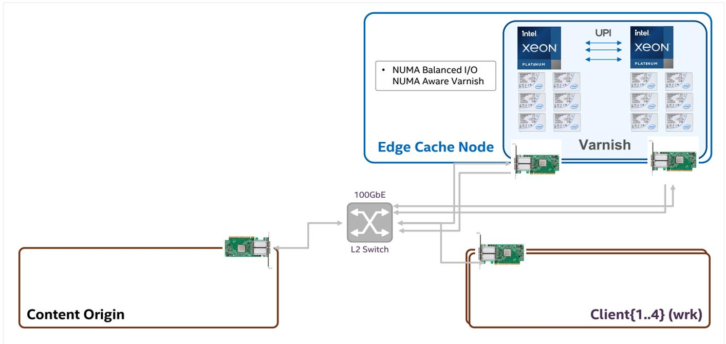
Figure 3. Dual-processor server CDN test setup
