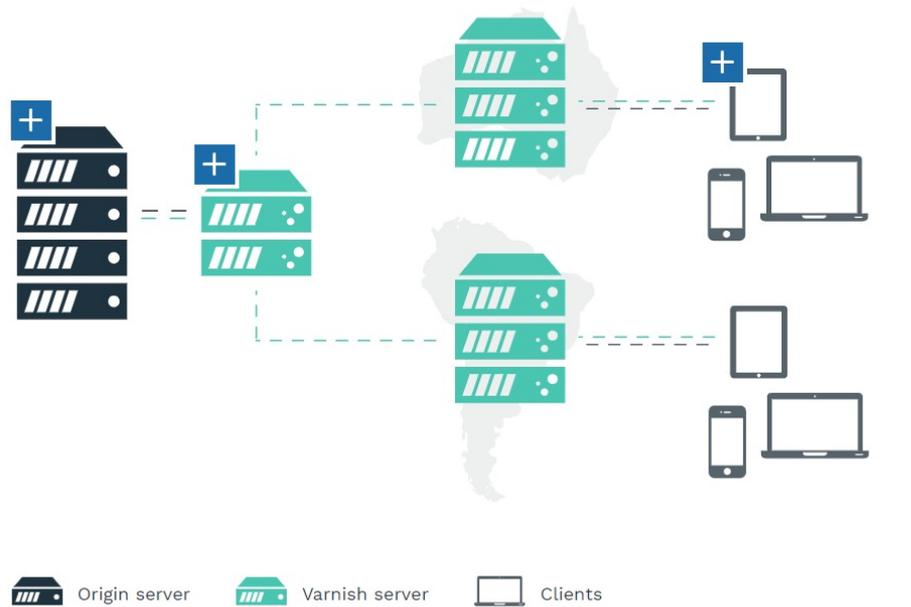
Figure 1. Two-tier Varnish solution architecture for a large-scale CDN.
