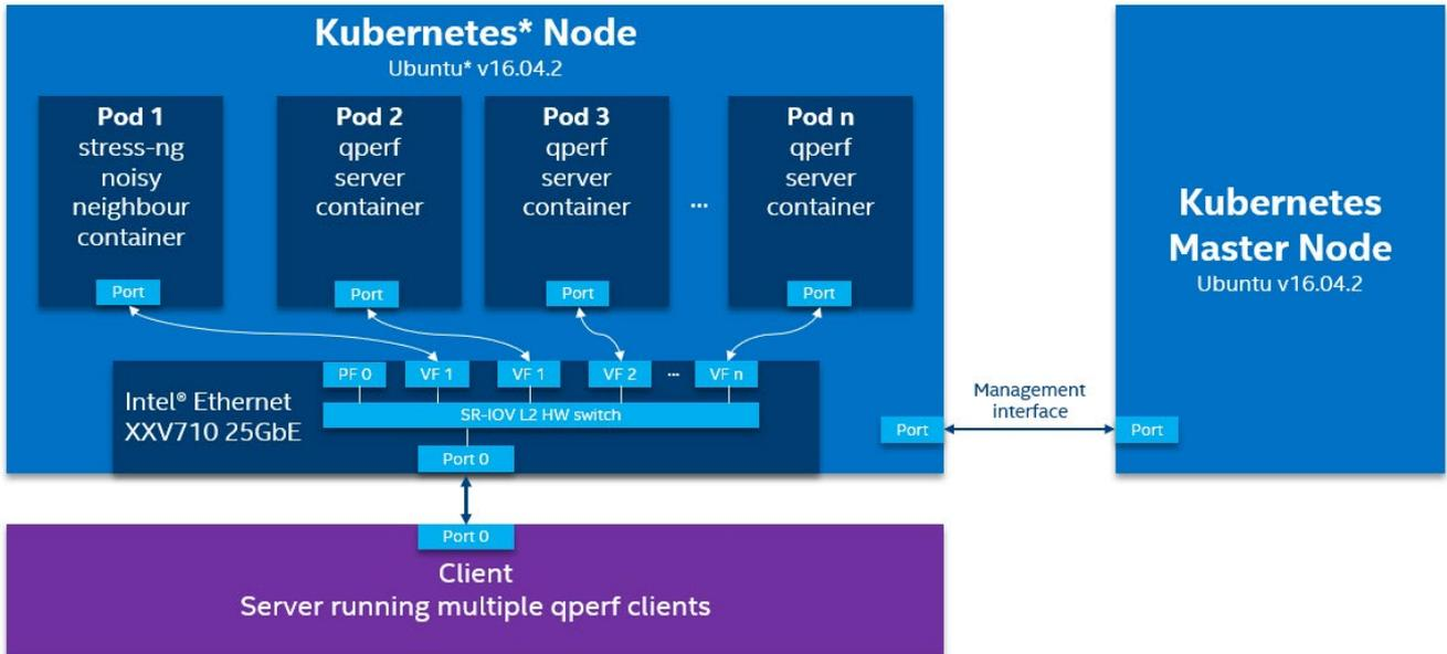
Figure 10. High-Level Overview of qperf Server Workload Setup
