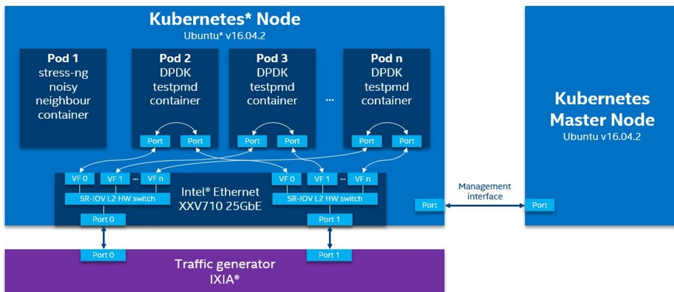
Figure 9. High-Level Overview of DPDK Testpmd Workload Setup<sup>2</sup>
