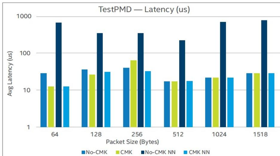
Figure 12. DDPK Testpmd Latency (lower latency is better)
