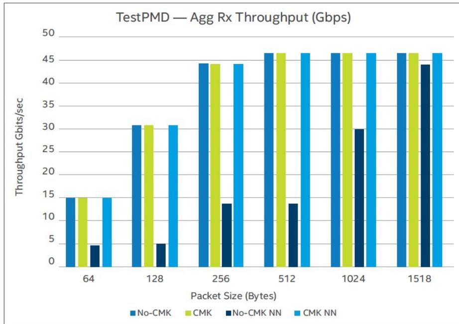
Figure 11. DDPK Testpmd Throughput (higher throughput is better)
