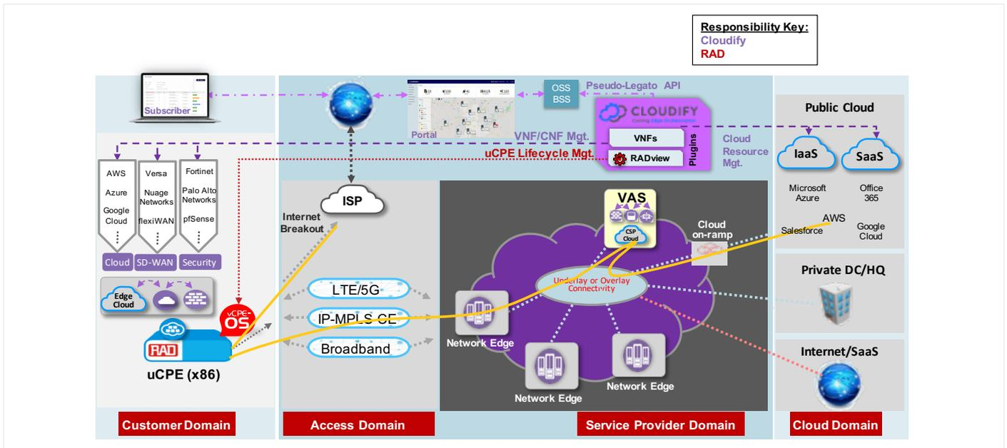
Figure 4. uCPE software stack secure device installation demonstration.
