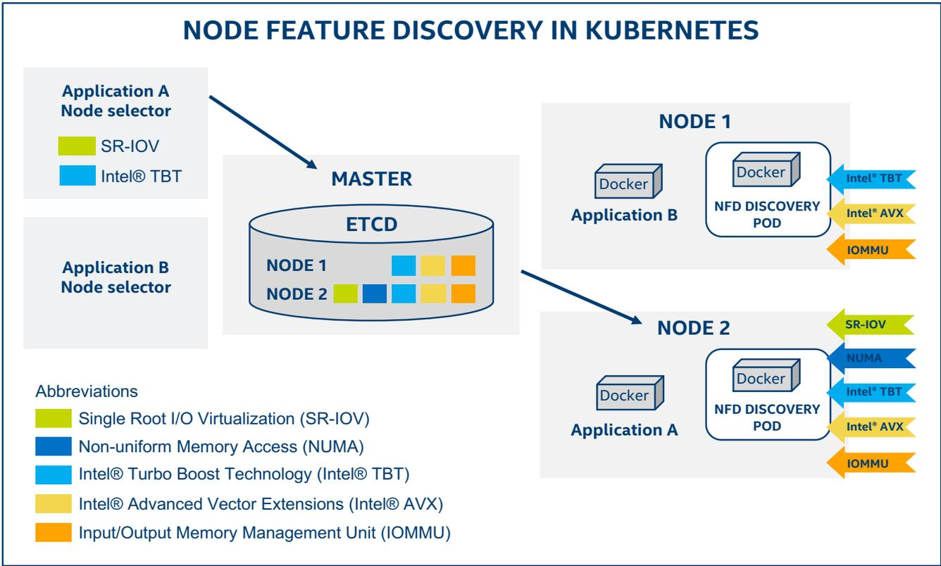
Figure 2. Utilizing NFD, each Kubernetes node is labeled with a list of the hardware capabilities it supports. In this figure, SR-IOV and NUMA are supported by Node 2, giving Node 2 an advantage for supporting performance sensitive workloads.
