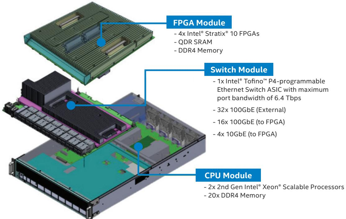
**Figure 4.** Interior of CASwell CAR-5056 with technology important to L4LB called out.
