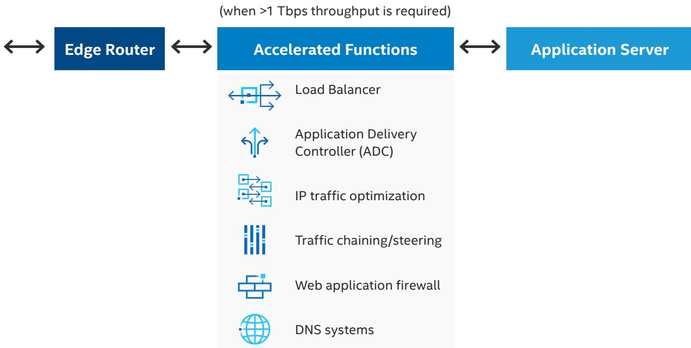
**Figure 1.** “Middle Box” network functions conceptual diagram with examples that can benefit from acceleration
