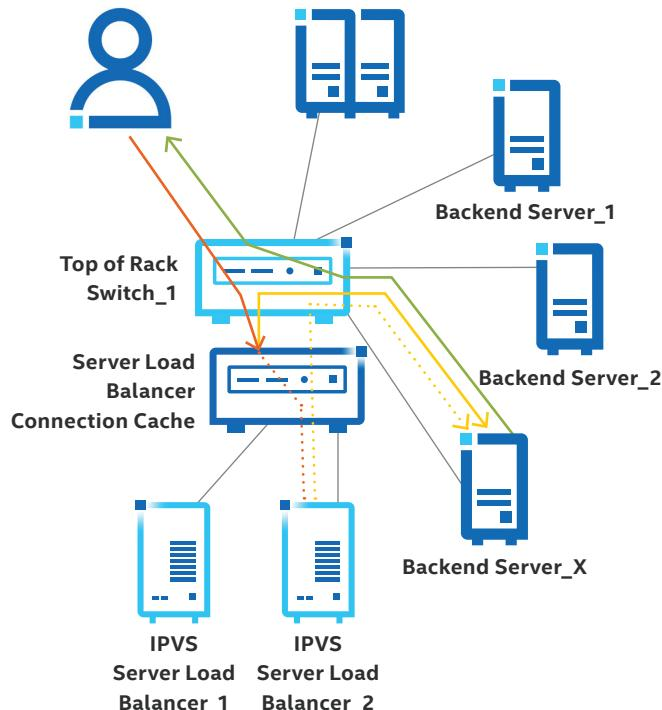
Figure 2. Example Load Balancer Architecture
