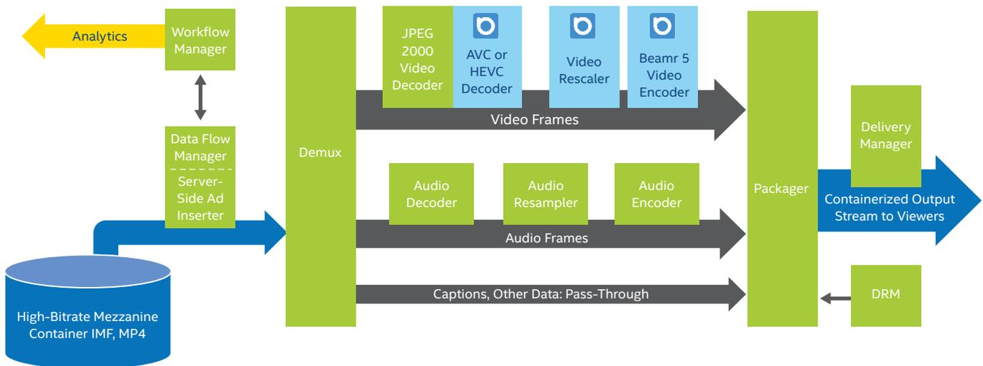
Figure 4. Origin transcoder (one of multiple instances running simultaneously).
