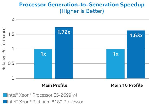
**Figure 3.** Beamr 5\* 4K HEVC encoder increased performance with the Intel® Xeon® Platinum 8180 processor.<sup>2</sup>
