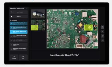
Digital Worker guidance system connected to ERP/MES/PLM to automatically enrich your work instructions with existing data
