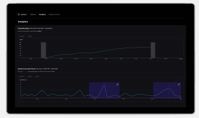
Data about error rates, cycle times and walking routes is collected for line balancing and continuous process improvement
