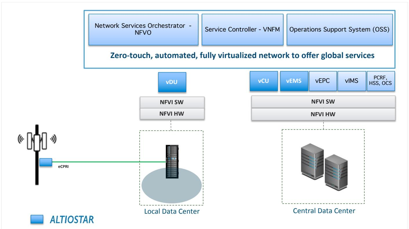
Figure 1. Model 1 diagram with vDU in a local data center that is served by a fiber-optic transport network.<sup>2</sup>
