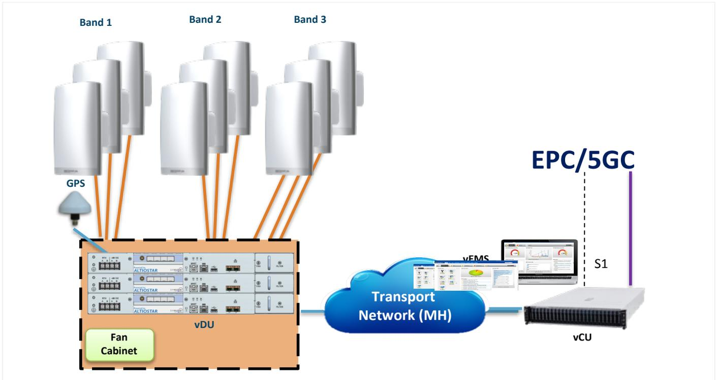
Figure 2. Higher performance server hosts vDU that can process data load of multiple RRHs.
