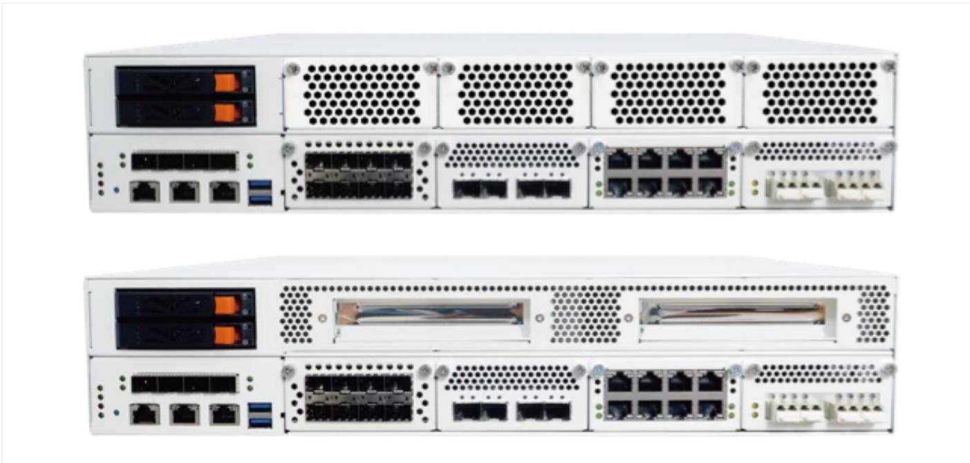
Figure 1. Front and back views of the AEWIN SCB-1921 MEC server.
