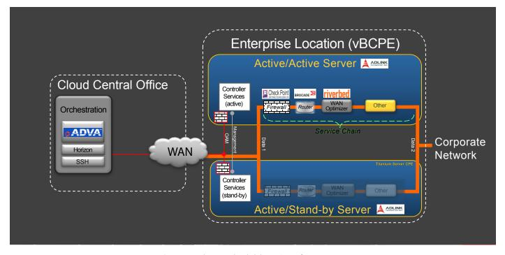
Figure 4: Wind River High Reliability vBCPE Reference Design
