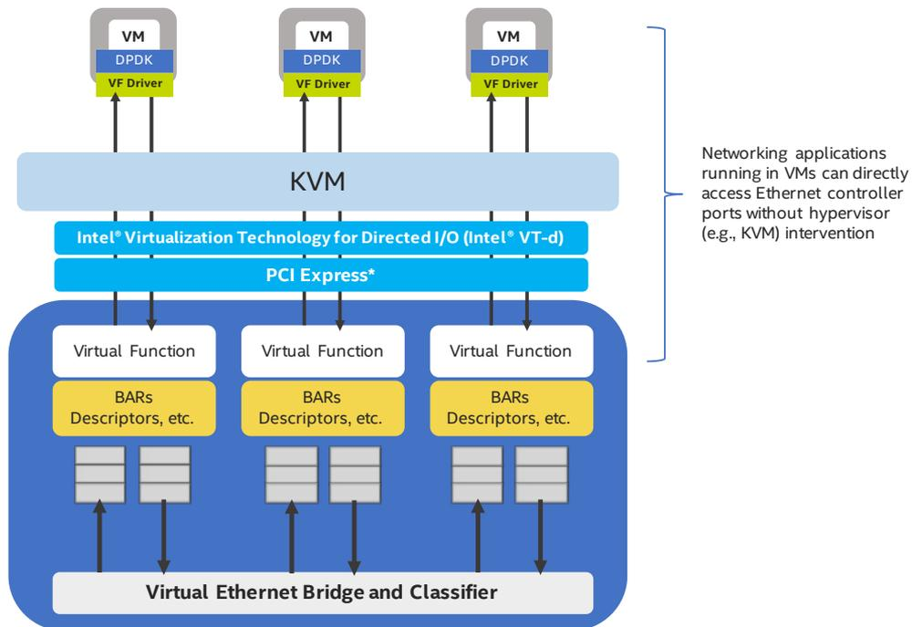
Figure 1. Example of KVM SR-IOV environment<sup>3</sup>
