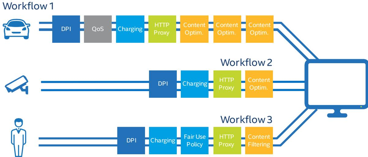
**Figure 4.** The Affirmed Services Workflow Orchestration framework enables fast and easy creation of services. QoS: quality of service, MVNO: mobile virtual network operator, Optim: optimization, Adapt: adaptation.
