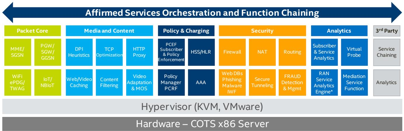
Figure 1. Solution architecture for Affirmed Networks\* Mobile Content Cloud\*.
