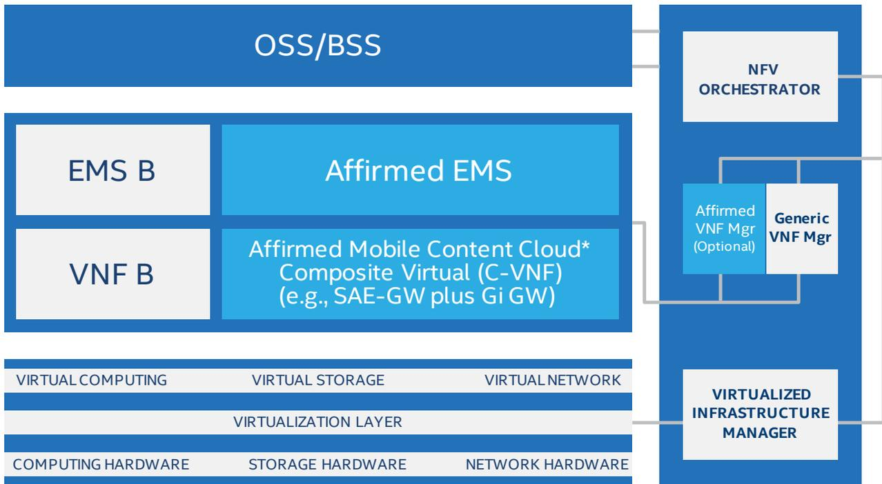
Figure 2. How Affirmed Networks\* Mobile Content Cloud\* fits into the framework. OSS/BSS: operations support system / business support system, EMS: element management system, VNF: virtualized network function.
