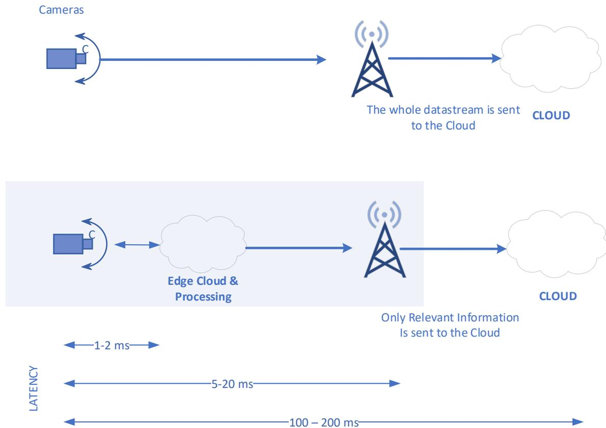
**Figure 5. High-level systems diagram of Stadium Edge Computing**
