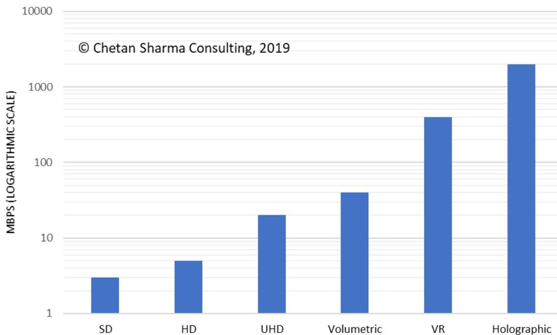
**Figure 7. Streaming requirements for different forms of media streaming**
