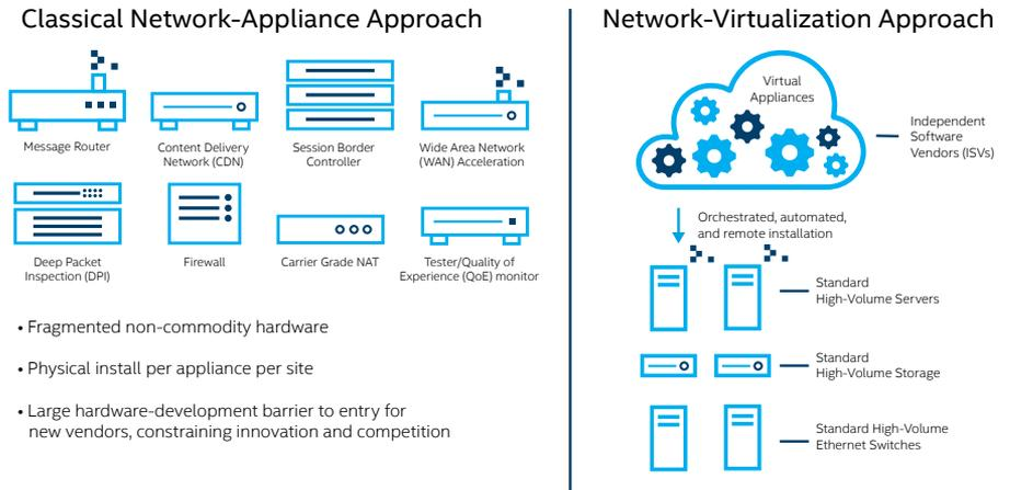
**Figure 1.** NFV allows for consolidation of multiple dedicated network appliances onto industry-standard, Intel® architecture-based servers, storage, and switches
