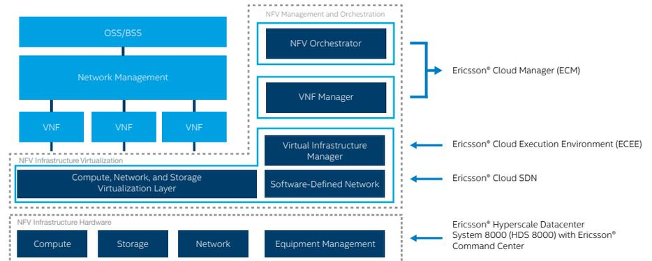
**Figure 3.** The Ericsson® NFVi with Ericsson® HDS 8000, based on Intel® technologies, provides orchestration between all roles defined by the ETSI model for NFV; the NFVi encompasses the hardware and software components found within the dashed line
