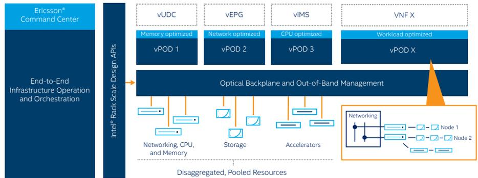
**Figure 5.** Ericsson® Command Center invokes Intel® Rack Scale Design APIs to compose vPODs from pooled resources; vPODs in the figure are running virtualized Ericsson® User Data Consolidation (vUDC), virtualized Ericsson® Evolved Packet Gateway (vEPG), and virtualized Ericsson® IP Multimedia Subsystem (vIMS)
