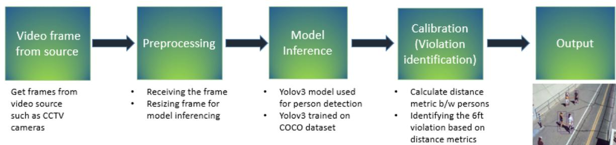
Fig 2 - Block Diagram of HCL's Social Distance Monitoring (SDM)
